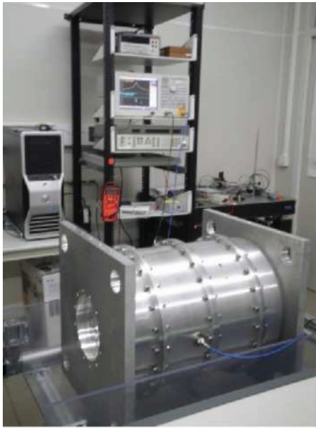
Figure 5: Cavity bead-pull test bench implementation.
