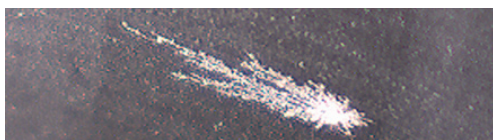
Figure 5: Tracks of arc damage, far from the high field region of the cavity. These tracks are 1 - 2 cm long.
