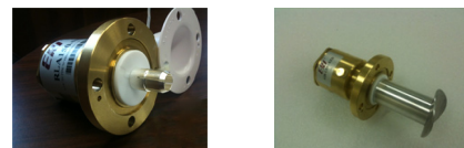
Figure 8: EIA connector and mock FPC probe showing coupler with inner conductor and “pringle” tip attached.
