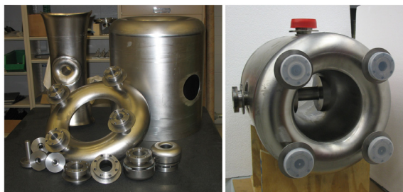
Figure 4: \beta = 0.53 HWR subassemblies (left) and a completed bare cavity (right)
