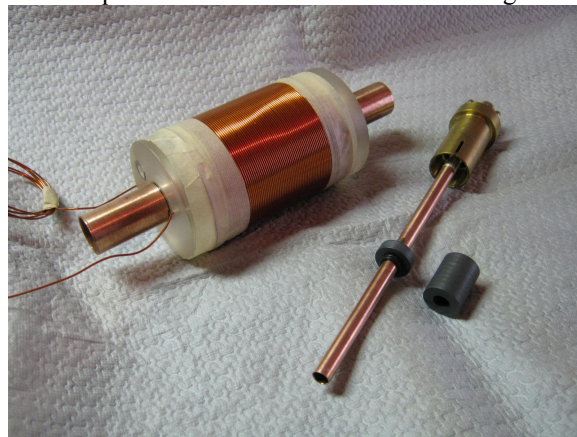
Figure 2: Solenoid test fixture, with ferrite on the center conductor of a 7 inch long coax.
