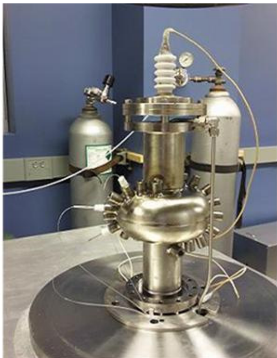
Figure 1: Specially designed perforated single cell cavity with optical fiber diagnostic tools.
