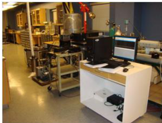
Figure 3: Complete system including RF power supply, vacuum system, bell jar assembly and diagnostic units.
