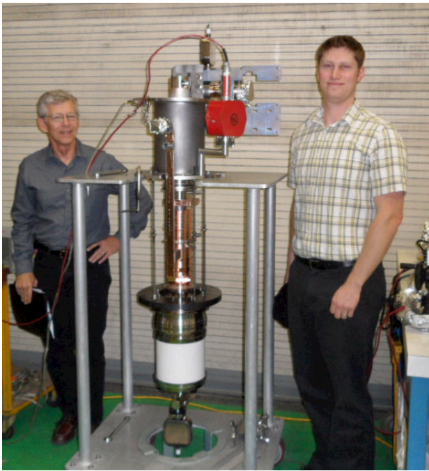
Figure 1. An XL-4 Klystron without solenoid.
