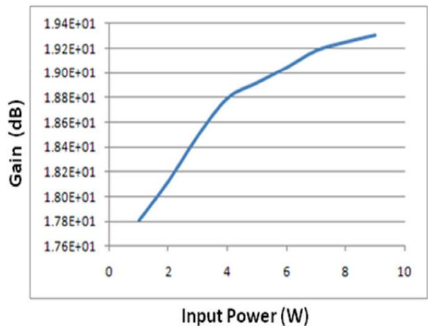
Figure 12: Measured gain of driver amplifier.
