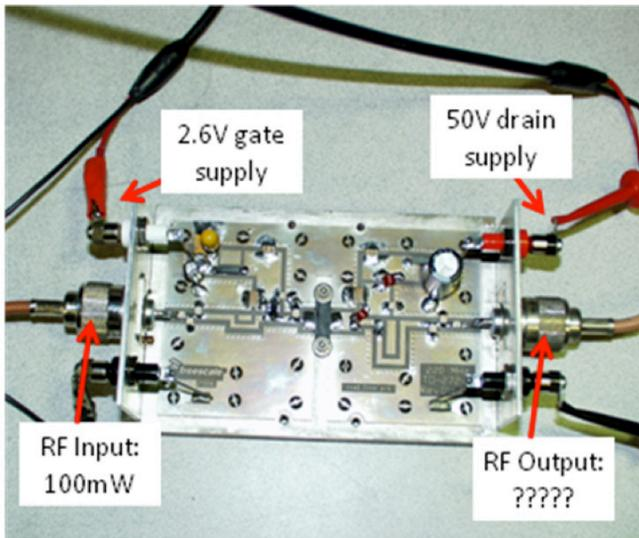
Figure 9: Driver amplifier connected to the test setup.
