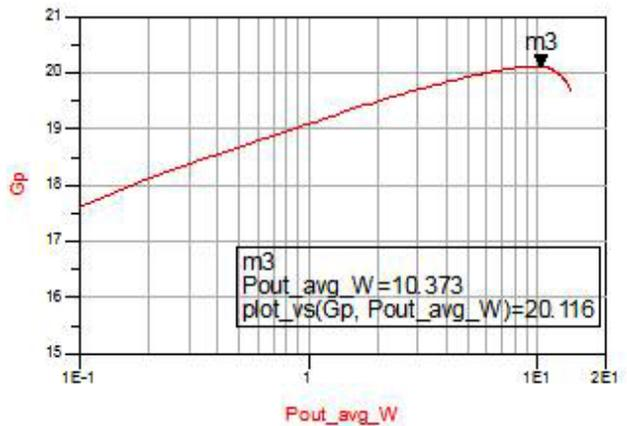
Figure 11: Simulated driver amplifier gain.
