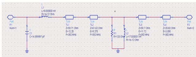
Figure 6: Output Matching Network for 450 MHz MRF6V2010N Driver.
