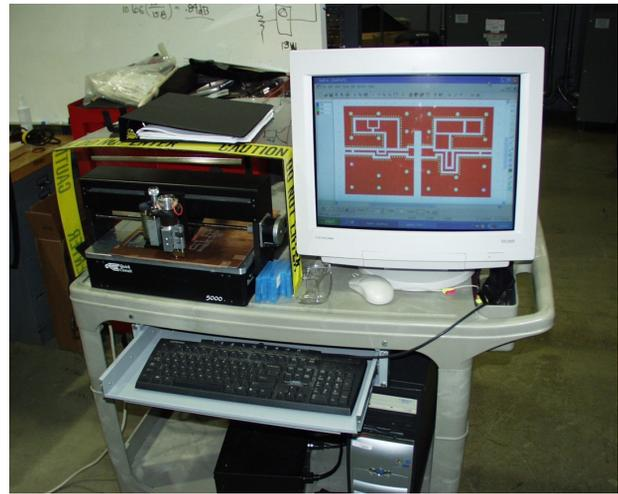
Figure 7: Quick Circuit 3000 prototyper.
