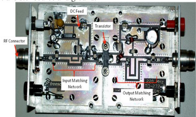
Figure 8: Prototype driver amplifier.
