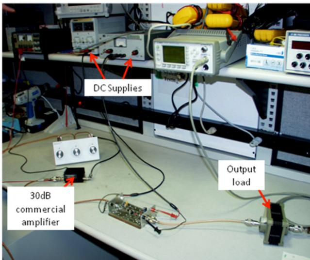
Figure 10: Driver amplifier test setup.
