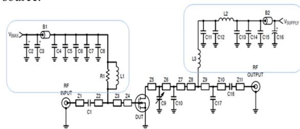
Figure 3: Driver circuit shown with DC networks circled.
