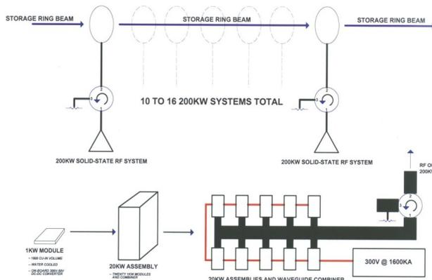
Figure 1: Proposed Solid State Amplifier System using 1kW Modules.
