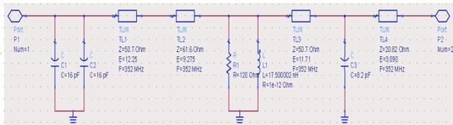
Figure 5: Input Matching Network for 450 MHz MRF6V2010N Driver.
