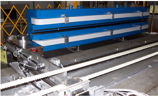
Figure 1: 35mm dipole prototype (Buckley).
