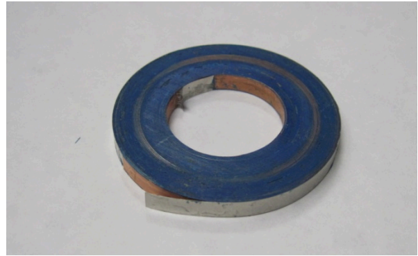
Figure 5: A picture of a test coil. The blue color is due to the epoxy used to fill small surface irregularities.
