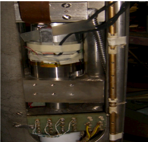
Figure 4: Photograph of the loading fixture showing the upper and lower jaws of the stress machine.
