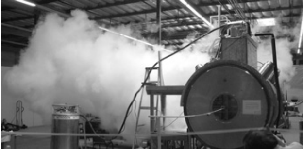
Figure 3: Quench during spectrometer solenoid training.
