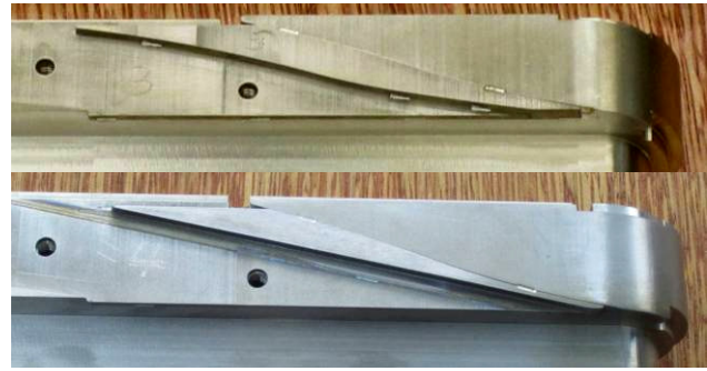
Figure 3: Two pictures from the Nose Piece before and after relaxing the bending radius.
