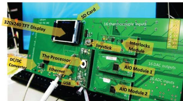
Figure 6: A 19" baseboard and full set of modules built for the IEX project development.
