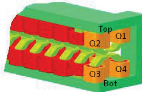
Figure 2: Downstream portion of the EMVPU prototype. Six trim coils are shown in orange.
