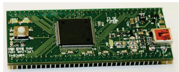
Figure 5: The ARM-based microcontroller.
