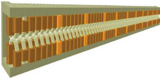
Figure 1: 38-period electromagnetic undulator.
