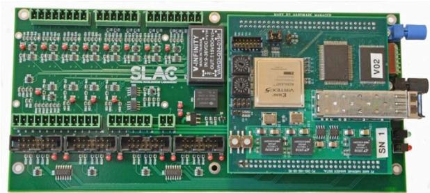
Figure 2: Hardware manager with Virtex board.
