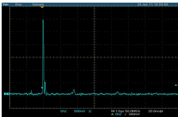
Figure 9: A reflection test with 100 ohm termination. 1.0  $\mu$ s per division. (Photo courtesy of FID GmbH)
