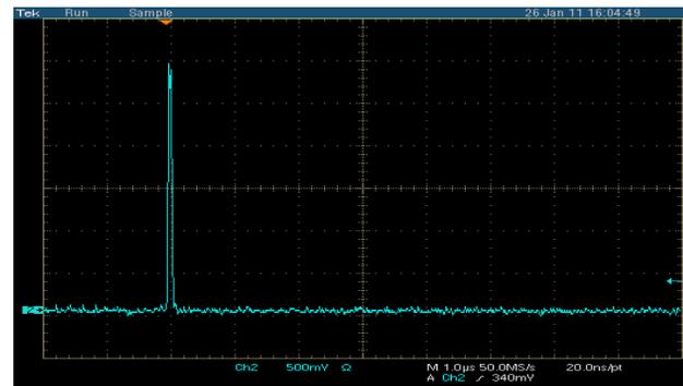
Figure 5: A reflection test with 18 ohm termination. 1.0  $\mu$ s per division. (Photo courtesy of FID GmbH)
