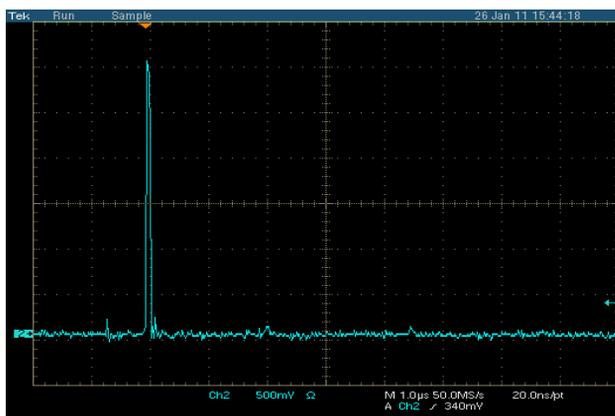
Figure 8: A reflection test with 75 ohm termination. 1.0  $\mu$ s per division. (Photo courtesy of FID GmbH)
