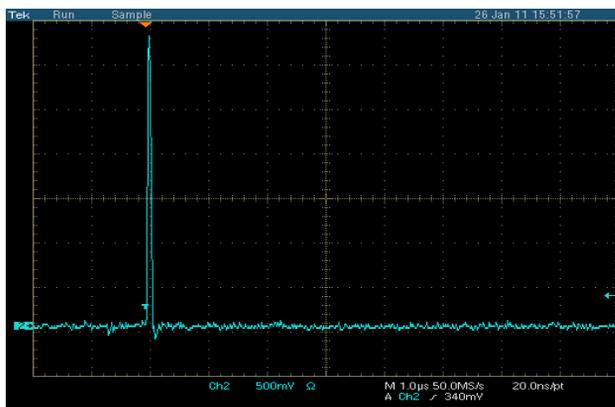
Figure 7: A reflection test with 50 ohm termination. 1.0  $\mu$ s per division. (Photo courtesy of FID GmbH)
