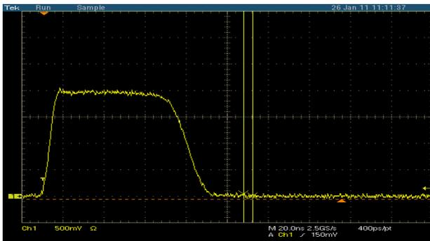
Figure 2: The output voltage waveform of FID Pulse Generator at 40kV. Vertical scale: 1:20,000, 0.5Vper division; Horizontal scale: 20 ns per division. (Photo courtesy of FID GmbH)
