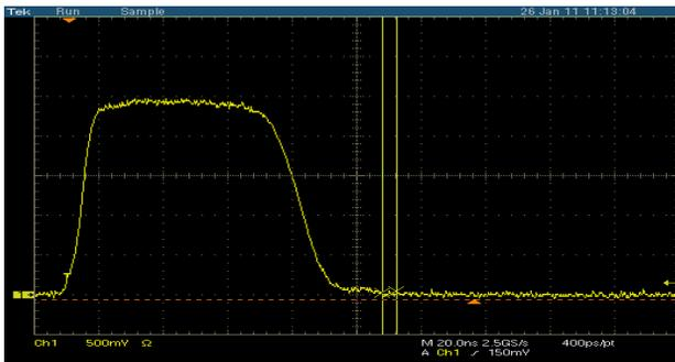
Figure 3: The output voltage waveform of FID Pulse Generator at 50kV. Vertical scale: 1:20,000, 0.5Vper division; Horizontal scale: 20 ns per division. (Photo courtesy of FID GmbH)
