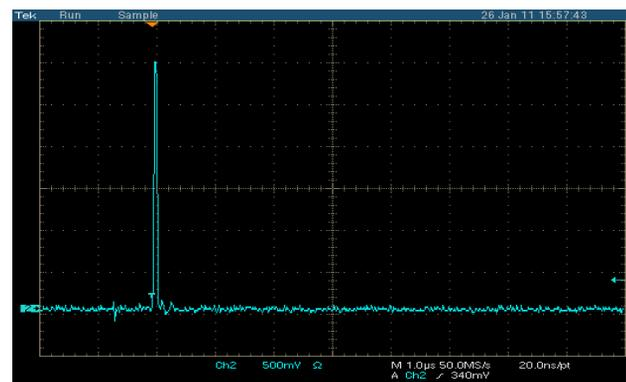
Figure 6: A reflection test with 27 ohm termination. 1.0  $\mu$ s per division. (Photo courtesy of FID GmbH)
