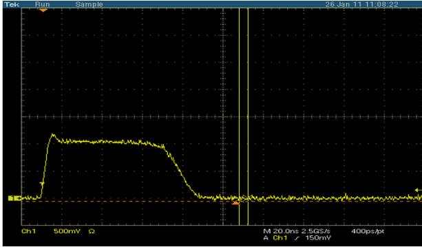
Figure 1: The output voltage waveform of FID Pulse Generator at 20kV. Vertical scale: 1:20,000, 0.5Vper division; Horizontal scale: 20 ns per division. (Photo courtesy of FID GmbH)
