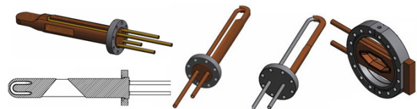
Figure 6: Models of photon absorbers (from left): crotch ABS, crotch ABS with zero opening, stick ABS with stainless cooling tube, and flange ABS.
