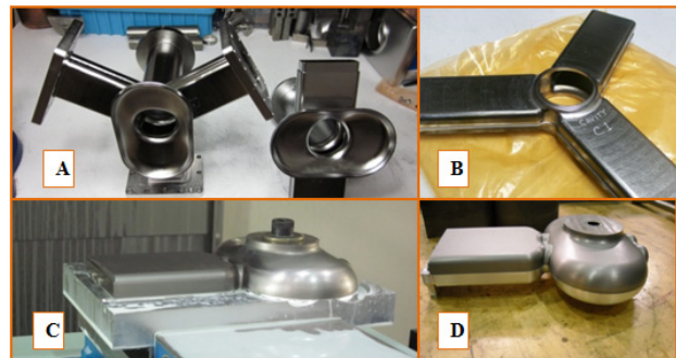
Figure 3: Bare crab cavity prototypes. A: two half CCB1 cavity groups before the final equator EBW; B: Y HOM waveguide group made by CNC machining for CCB1 cavity with RRR>250 Nb; C: CCA2 cavity fabricated on CNC machine; D: Finished Nb and Al prototype cavity.
