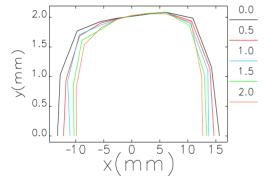
Figure 3: Dynamic aperture at  $\delta = -2.5\%$  when the multipole errors listed in Table 1 and 2 are multiplied by a factor of 0,0.5,1.0,1.5, and 2.0, respectively.
