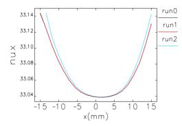
Figure 2: Amplitude-tune dependence at  $\delta = -2\%$
