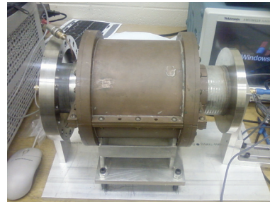
Figure 1: The WGM on the test bench. A thin metallic wire passes through the WGM, with one end connected to the function generator and the other end terminated by a 50 Ω terminator. The output signal is measured by an oscilloscope.
