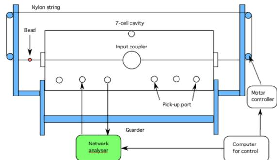
Figure 1: Electromagnetic field measurement using bead-pull method and network analyzer.
