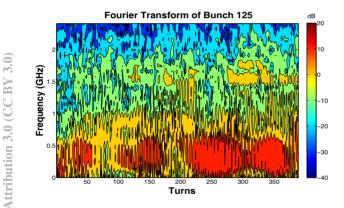
Figure 3: Spectrum at E-cloud motion shows primary content below 500 MHz and relaxation oscilations.
