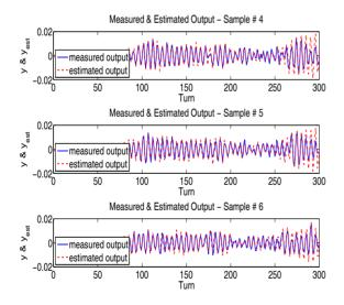
Figure 7: Results show that vertical displacements for different longitudinal bunch slices can be recovered using identification methods for time varying system.
