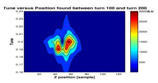
Figure 1: Tune Shift of the Bunch tail about the nominal value of 0.185 due to E-Cloud.
