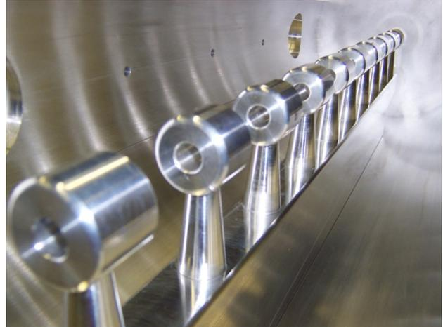
Figure 3: A close-up view of the DTs mounted on the vane in the bottom part of the cold-model assembly.
