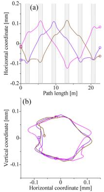
Figure 4: (a) Single-particle orbits of the beam in Fig. 3 while the beam circulates the storage ring once. The horizontal orbits of three ions arbitrarily picked out from the ordered beam are shown. The six gray shaded areas indicate the bending-magnet sections. (b) The trajectories of the three ions in the cross-sectional view are shown. In both panels, the square and circle symbols represent the initial and final coordinates of the ions during one turn, respectively.
