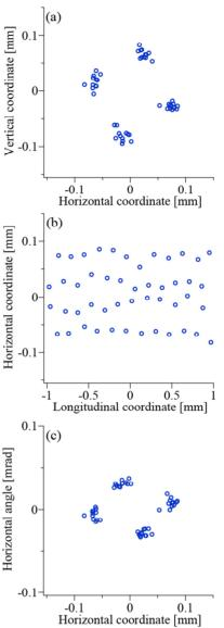
Figure 3: Real-space and phase-space configurations of the laser-cooled beam in Fig. 2. Each blue circle corresponds to a single  $^{24}Mg^+$  ion.
