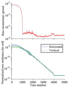
Figure 2: Time evolution of the longitudinal momentum spread and transverse emittance of the 40-keV  $^{24}Mg^+$  ion beam during laser cooling. The bare betatron tune  $v_0$  is 1.44. The line density of the beam is  $2.4 \times 10^4$  m<sup>-1</sup>. The laser detuning is scanned in 1000 turns. The horizontal displacement and final detuning of the lasers are 3 mm and -81 MHz, respectively.
