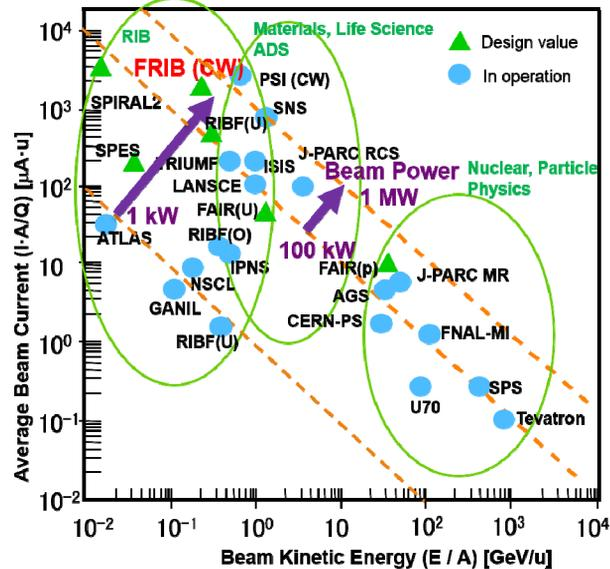
Figure 1: Average beam power as a function of the kinetic beam energy for various operating and proposed proton and heavy-ion accelerator projects.
