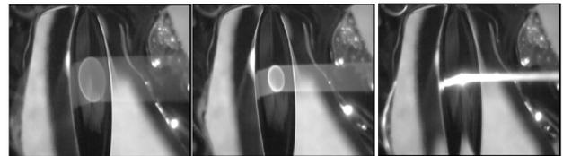
Figure 3: Liquid lithium film flowing at high speed ( $\sim 50$  m/s) intercepting a proton beam of about 60 kV at ANL. The test produced power deposition densities similar to the FRIB uranium beams.
