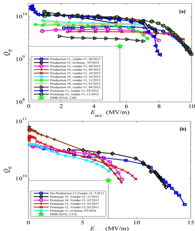
Figure 4:  $Q_0$  vs.  $E_{acc}$  performance tested at 2 K for (a)  $\beta_0=0.085$  QWR prototypes used in the ReA3, and (b) the prototype and pre-production  $\beta_0=0.53$  HWR.
