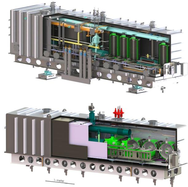
Figure 5: FRIB “bottom-up” cryomodule designs. The top cryomodule contains 8  $\beta_0=0.085$  QWRs, 3 solenoids, and 3 cold beam position monitors; the bottom cryomodule contains 8  $\beta_0=0.53$  HWRs and a solenoid.
