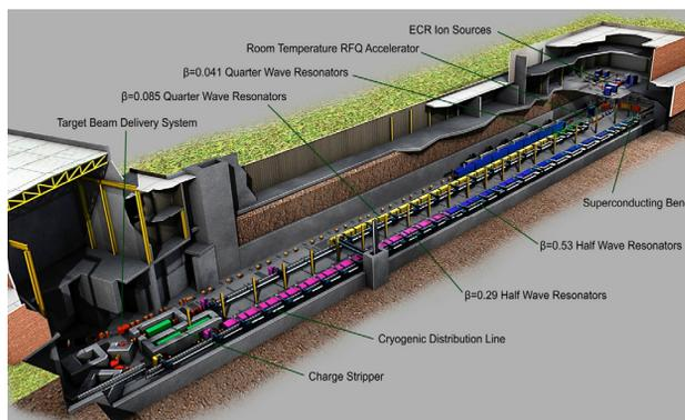
Figure 2: Layout of the FRIB driver accelerator.
