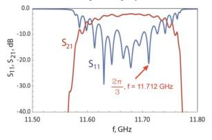
Figure 4: Transmission and reflection through the assembled 16 cell PBG structure.
