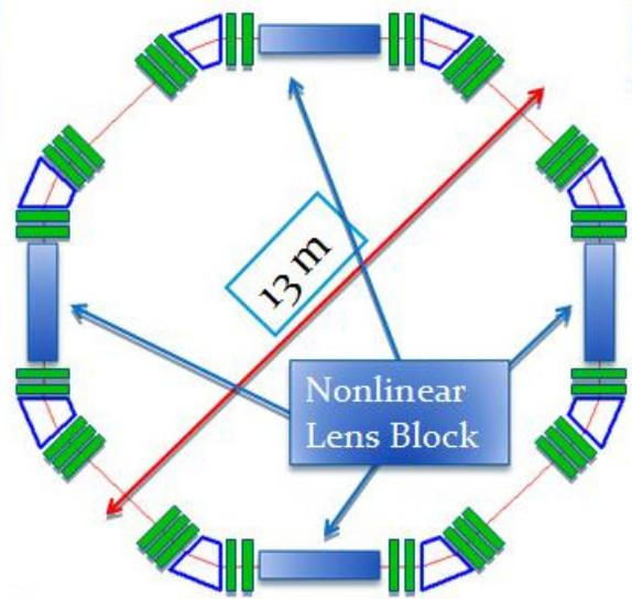
Figure 3: Schematic of storage ring with a nonlinear close to integrable focusing system from [2].
