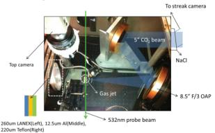
Figure 1: Experimental setup in the target chamber.
