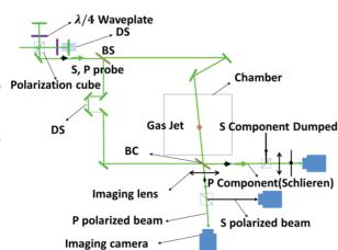
The two-frame polarization based interferometry and schlieren optical scheme is depicted in Fig. 3.
