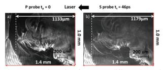
Figure 4: Two-frame interferogram at different times. a) shows P probe. b) shows S probe with 46ps delay. White dashed line shows the instantaneous position of the overdense plasma layer pushed by the radiation pressure.
