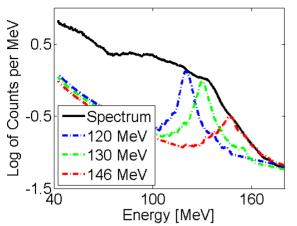
Figure 2: Process of comparing the rotated and linearized transverse lineouts (dashed lines) against the central lineout of the electron spectrum (solid black line). The converted transverse lineout at 146 MeV (red dashed curve) is asymptotic with the central lineout; therefore the maximum electron energy is 146 MeV.
