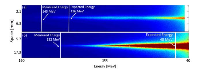
Figure 3: (a) Typical low-density electron spectrum. The cell length  $l_{cell}$  was 1100  $\mu$ m, the plasma density n was 9.1 x  $10^{18}$  cm<sup>-3</sup>, and  $a_0$  was 2.00. (b) Typical high-density spectrum.  $l_{cell}$  was 430  $\mu$ m, n was 2.2 x  $10^{19}$  cm<sup>-3</sup>, and  $a_0$  was 1.86.
