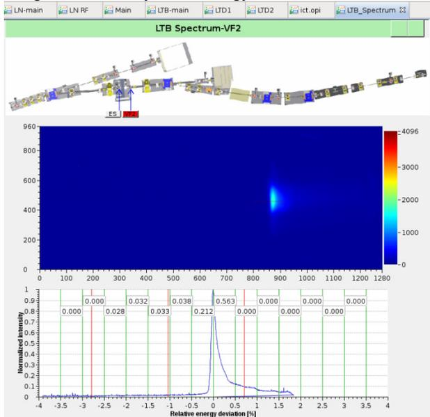
Figure 1: Screenshot of beam energy and energy spread measurement with flag VF2 in LTB transport line.
