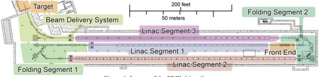
Figure 1: Layout of the FRIB driver linac.
