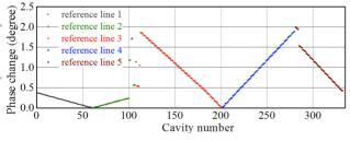
Figure 5: Phase change ("degree" corresponds to the cavity rf frequency) for each of the cavity along the linac.
