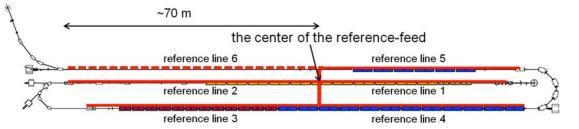
Figure 3: Schematic layout of the reference lines and the center of the reference-feed in the linac tunnel.
