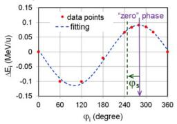
Figure 2: Phase scan of a  $\beta$ =0.041 QWR with uranium beam (q/A=33/238) at 0.5MeV/u to set the synchronous phase of the cavity.
