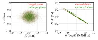
Figure 6: Sampled particle distributions on target with (in red) and without (in green) the phase changes. Both transverse (left) and longitudinal (right) are very similar for the two cases.
