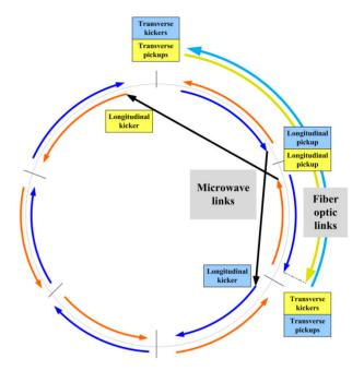
Figure 1: Locations of pickups and kickers (blue and yellow boxes), longitudinal system microwave links (black arrows), and transverse system fiber optic links (light blue and yellow arrows). The dark blue and orange arrows indicate the directions the beams travel.
