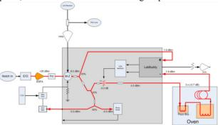
Figure 9: One-turn delay notch filter block diagram. The input from the microwave link is at the top. The block on the left labelled "Notch In" is for the network analyzer measurements. The output at the right of this diagram is connected to the input of the signal fanout.
