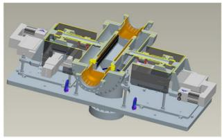
Figure 4: A cross-sectional view of the horizontal pickup vacuum chamber and assembly.
