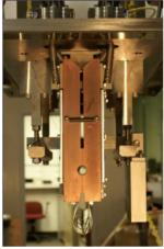
Figure 6: Photographs of the first Blue vertical kicker cavity assembly that used the scissor design, in the open position (left) and the closed position (right). The aperture in the closed position is 2 cm.
