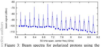
Figure 3: Beam spectra for polarized protons using the keyhole longitudinal pickup. The traces are centered at 5.8, 6.0, ..., 9.0 GHz and each have a 50 kHz span.
