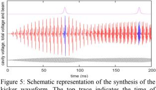
Figure 5: Schematic representation of the synthesis of the kicker waveform. The top trace indicates the time of arrival of two bunches at the kicker. The bottom trace indicates the voltage present on a single kicker cavity, and the middle trace indicates the sum of the voltage on the 16 cavities (red). The blue sections of the middle trace indicate the desired broadband kicker waveform.
