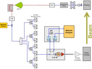
Figure 8: Electronics block diagram for one of the transverse systems. Red lines indicate fiber optic signal paths; blue lines indicate electrical signal paths.
