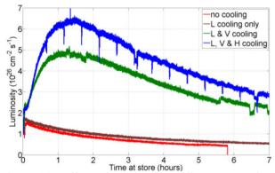
Figure 10: Effect of stochastic cooling on Uranium-Uranium luminosity.
