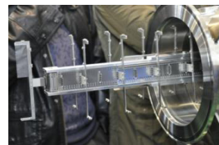
Figure 11: Stripping foil for H - injection.
