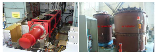
Figure 7: 3MW klystron and its 120 kV HVPS under manufacture.
