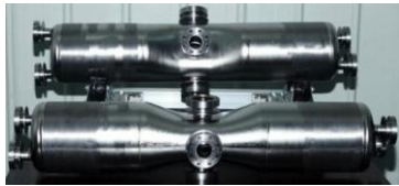
Figure 17: Prototype QWR cavity with \beta=0.1 for Injector-II.
