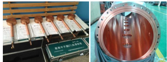
Figure 6: The fabricated drift tubes and tank.
