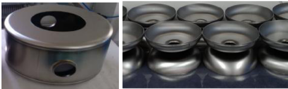
Figure 18: Prototype development of 325 MHz spoke cavities with \beta = 0.21 and some 650 MHz elliptical cavities with \beta = 0.82 , for main linac.
