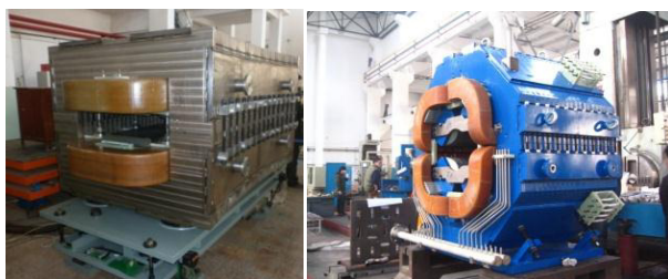
Figure 8: RCS dipole and quadrupole magnets in mass production.
