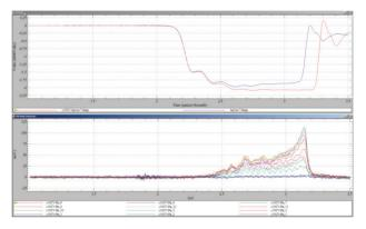
Figure 6: Injector voltage waveforms. Top waveform showing normal (red) and droop (blue) conditions. Bottom waveform shows PIN diode signals recorded during injector voltage droop.
