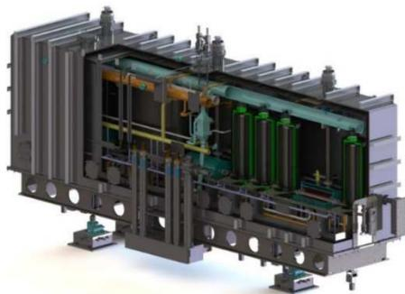
Figure 1: Cross-Section of ReA6  $\beta=0.085$  QWR Cryomodule.
