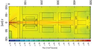
Figure 1: Proton flux seen in the first three quadrupoles of the fragment selector at FRIB. The figure is from ref [2].
