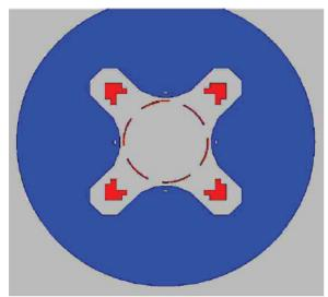
Figure 4: Sketch of the sextupole coils inserted into the BNL R&D quadrupole magnet.
