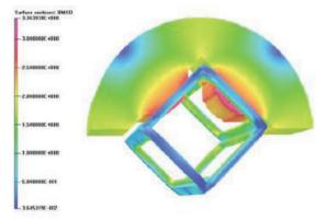
Figure 2: Opera 3D magnetic model of the FRIB fragment separator quadrupole. The sketch shows all of the coils and the upper half of the yoke.
