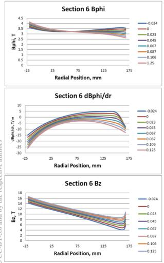
Figure 5:  $B_{\phi}$ ,  $dB_{\phi}/dr$ , and  $B_z$  vs. r for section 2. The different colors represent different ellipse asymmetries.
