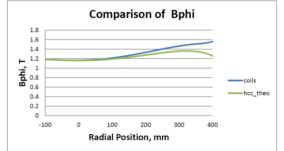
Figure 4: Comparison of the coil description of  $B_{\phi}$  with the theoretical Bessel function description for section 2.
