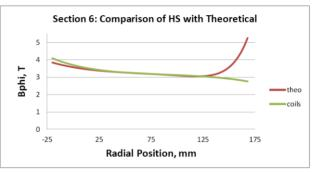
Figure 7: Comparison of  $B_{\phi}$  calculated from the Bessel function description with that from HS coils.
