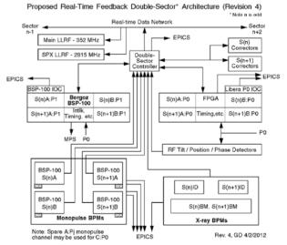
Figure 1: Real-time feedback double-sector controller architecture.
