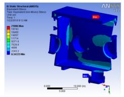
Fig. 6: Stresses on the vacuum Chamber.
