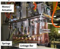
Fig. 3: Scissor Like Actuator.
