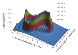
Figure 3: Heat input of 111 bunches of  $0.7 \cdot 10^9$  Au ions with an emittance of  $4\pi$  mm mrad on the beam dump window, with an additional vertical kicker.
