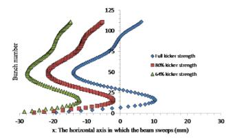
Figure 1: Kicker pulses for full kicker strength, and reduced strengths of 80 and 64 percent.
