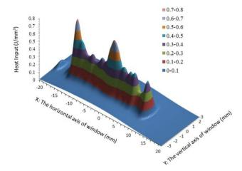
Figure 2: Heat input of 111 bunches of  $0.7 \cdot 10^9$  Au ions on the beam dump window, assuming a 95 percent normalized emittance of  $4\pi$  mm mrad.
