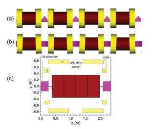
Figure 2: Cooling scheme for the Muon Collider. Fig. (c) depicts one lattice cell. The tilts of the magnets are not shown.
