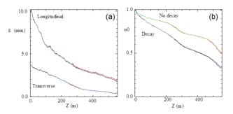
Figure 4: ICOOL and Warp cross-check without space charge (a) emittance, and (b) number of muons. Simulations are carried with and without muon decay using both codes.
