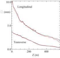
Figure 6: Beam normalized rms emittances along the channel with (red) and without (black) space-charge.
