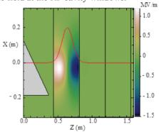
Figure 5: Longitudinal electric self-field. The red curve shows the scale current to show the location of the beam bunch.
