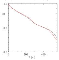
Figure 7: Fraction of beam remaining with (red) and without (black) space-charge.
