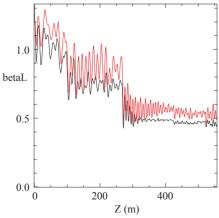
Figure 8: Longitudinal beta function with (red) and without (black) space-charge.
