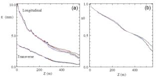
Figure 9: Emittances with varying RF gradients. The emittance is reduced with each 1.5 MV/m increment. The black curve, without space charge, is for reference. (b) Fraction of beam remaining for varying RF gradients. The black curve, without space charge, is for reference.
