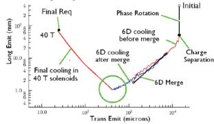
Figure 1: Baseline cooling requirement for the Muon Collider
