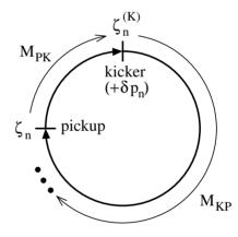
Figure 1: Schematic plot of the one turn transformation of the betatron state-vector in a lattice with damper.
