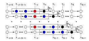
Figure 3: Schematic diagram representing the work of digital filter for K turns with single erroneous measurement ((-d)-th turn shown with a red circle).
