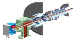
Figure 4: Input coupler assembly.
