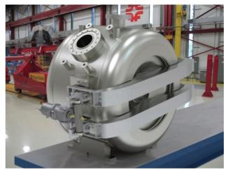
Figure 3: Dressed cavity and tuner.
