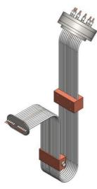
Figure 5: Conduction cooled current lead assembly.
