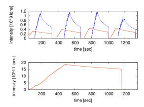
Figure 3: Comparison of the lifetime performance of typical Au-Au stores at 2.5 GeV/n in the Blue and Yellow ring (top) with a typical proton store at 5.86 GeV (bottom) in the Yellow ring
