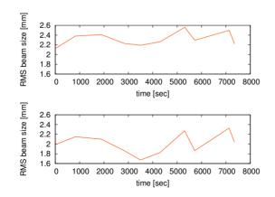
Figure 6: RMS beam sizes measured by using the RHIC polarimeter target as a wire scanner during the dynamic aperture studies
