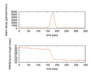
Figure 5: Hourly beam decay (top) and average bunch length during the dynamic aperture measurement using transverse emittance blow-up via the RHIC tunemeter
