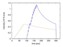
Figure 2: A typical Au-Au store at 2.5 GeV/n beam energy during a test run in 2012. While 27 bunches are being injected into the Blue ring, the intensity in the Yellow ring decreases by some 25 percent due to the short beam lifetime.
