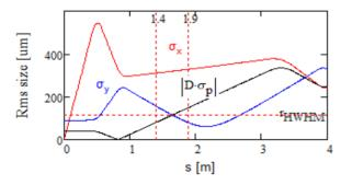
Figure 4: Rms beam sizes (horizontal  $-\sigma_x$ , vertical  $-\sigma_y$ , and due to momentum spread  $-|D\sigma_p|$ ) in vicinity of cooling chicane starting from the center of OSC section. Vertical lines mark location of wiggler. The horizontal line shows diffraction limited spot size (HWHM) of amplified radiation in the kicker wiggler.
