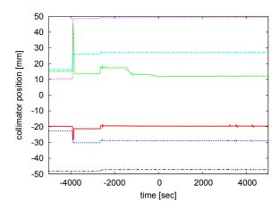
Figure 3: Recorded RHIC collimator positions during the beam experiment. The vertical collimator (green line) reached its final position at 11.5 mm. The horizontal axis is consistent with the one used in Figure 4.
