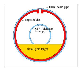
Figure 2: Schematic drawing of the proposed STAR internal target (Not to scale). The target will be installed at a distance of 2 m from the interaction point in the 3 inch inner diameter beam pipe. The aperture of the target is chosen slightly smaller than the 40 mm ID detector beam pipe.
