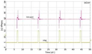
Figure 4: 80 kHz modulator test with beam-current pulse (red), and the anode-voltage pulse (yellow).
