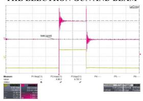
Figure 2: Example of the measurements of the 1085 mA current of the electron beam (yellow) and the anode voltage (red).
