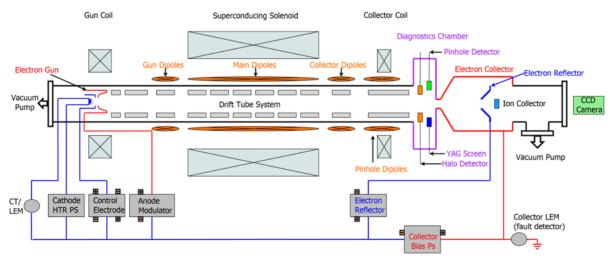
Figure 1: Layout of the electron lens test bench.
