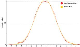
Figure 7: Beam profile from YAG screen, showing the correspondence between the experimental and fitted data.
