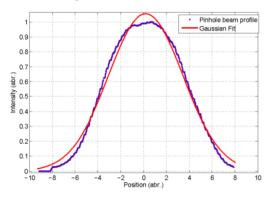
Figure 6: Beam profile obtained using pinhole scanner.
