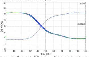
Figure 5: Rise and fall times of the electron beam measured via the anode voltage.
