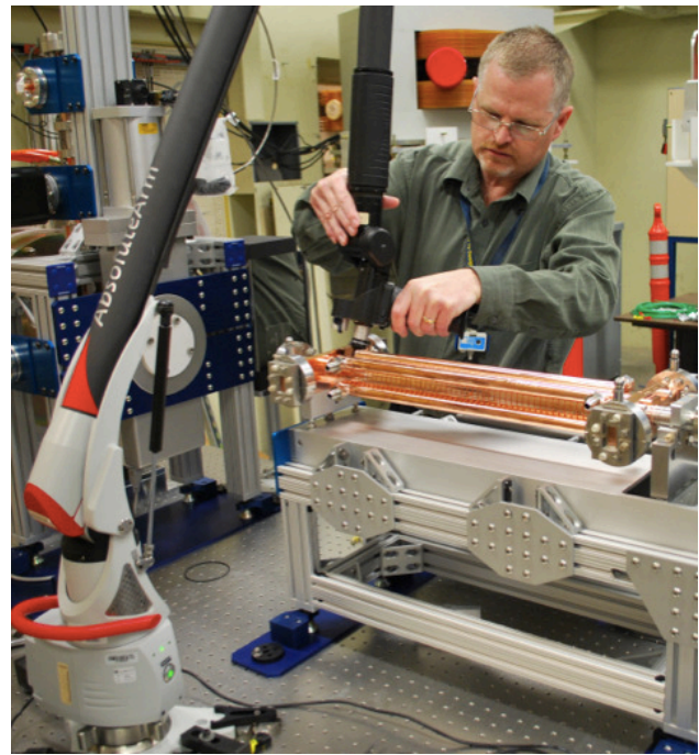
Figure 3: Photograph of X-band test station alignment. Romer CMM arm in use to precisely measure the 3D position of the T53 cells for proper alignment of the accelerating structure with respect to the beamline axis and cathode position.
