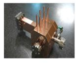
Figure 4: Structure of 2 cell rf-deflector.
