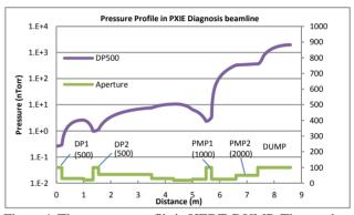
Figure 4: The pressure profile in HEBT-DUMP. The number in parentheses is pumping speed in l/s. there is no gas flow at the ends.
