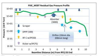
Figure 3: The pressure profile in MEBT. There is no gas flow at the both ends. The number in parentheses is pumping speed in l/s.
