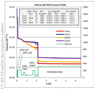
Figure 2: The pressure profile in IS-LEBT-RFQ. The number in parentheses is pumping speed in l/s. The IS has 1000 l/s turbo in its upstream chamber and 2000 l/s in down stream chamber. The flow rate of hydrogen is 0.5
