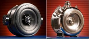
Figure 9: SSR1 cavity, bare (left) and dressed (right).
