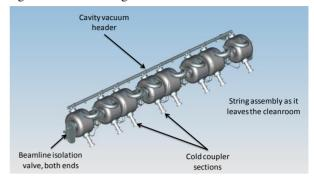
Figure 8: The SSR1 cavity and solenoid string assembly.
